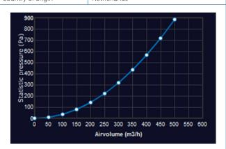
Air volumes are mentioned per filter cylinder. Recommended maximum output per cylinder is 156 m³/h.
